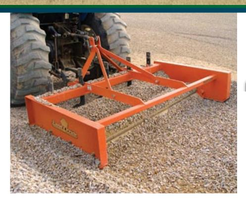
The **Grading Scraper** is ideal for renovating gravel driveways and roads, leveling construction and turf sites, and cleaning barns and chicken coups.
